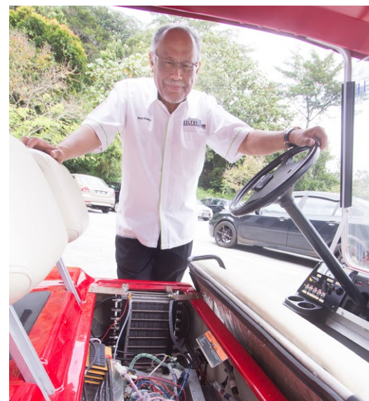
Two UKM-made 1.5 kW PEM fuel cells stacks underneath the seat of UKM's fuel cell golf cart
