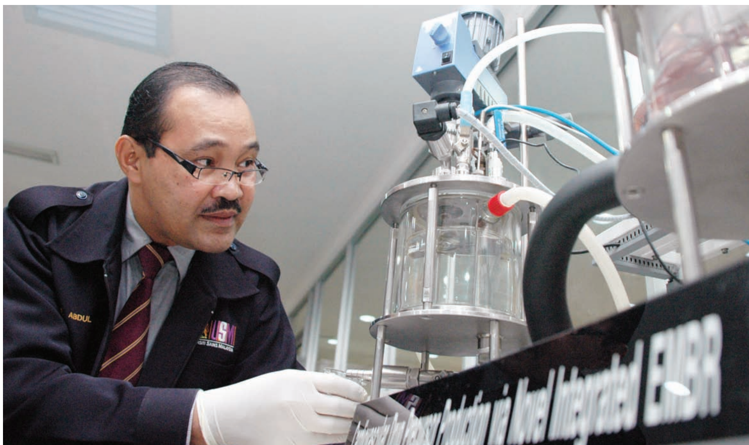
Prof Latif working with Enzymatic Membrane Bioreactor (EMBR) Producing Drug Precursors
